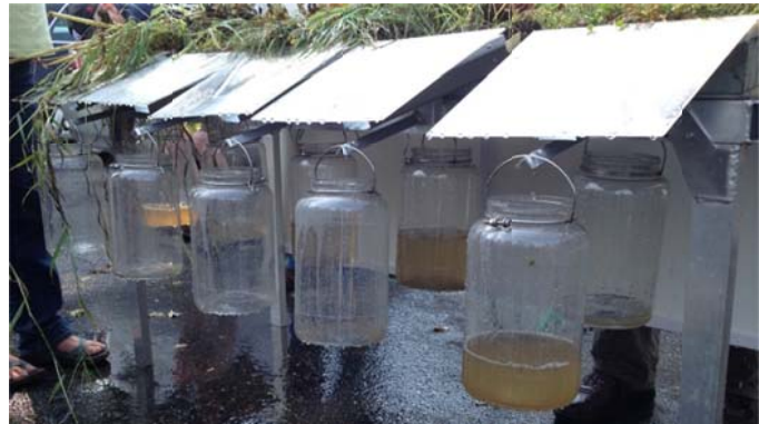
Figure 7 Rainfall simulation showing how water sinks into, or flows off, soils under different management styles. Note the two rotated pasture samples (2nd and 3rd from right) vs. continuously grazed soils (right).
